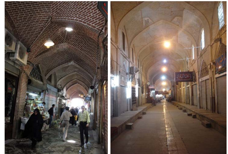
Figure 5: Bazaar of Tabriz with relatively short vaults (left) as opposed to Vakil bazaar in Shiraz (right) with very high vaults
