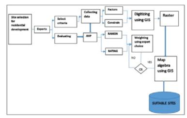
Fig.3: GIS modelling process for suitable site selection
